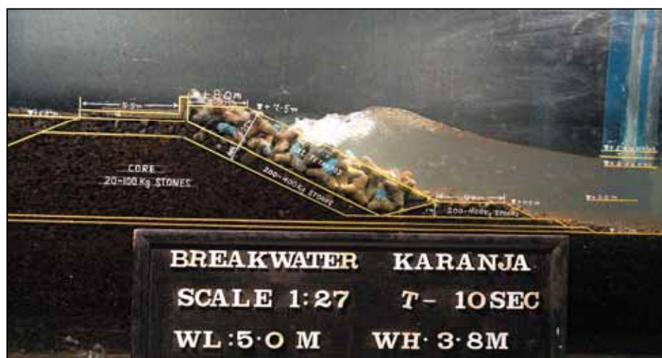
Wave Action at Breakwater During Flume Studies
