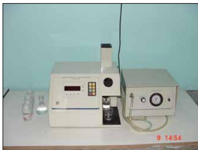
Estimation of Metal Ions in Water and Sediment Extracts Using Flame Photometer
