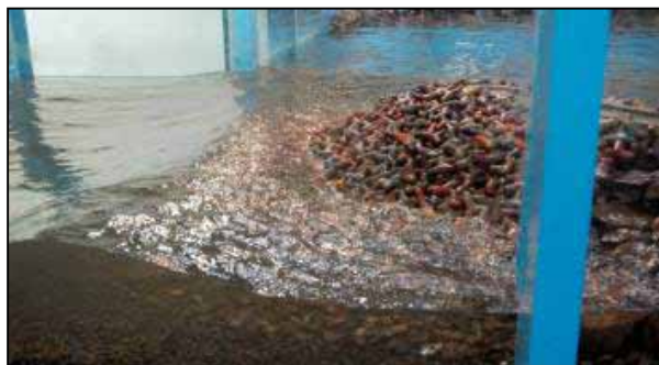
Wave Attack on Roundhead Portion of Breakwater in 3-D Diffraction Basin
