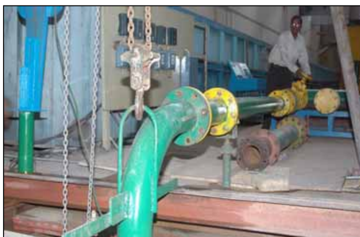
Submersible Pump Installed in Test Rig
