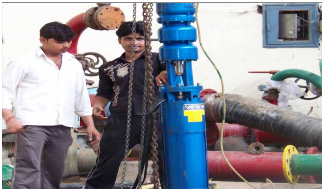
Submersible Pump Being Lowered in Pump Test Rig
