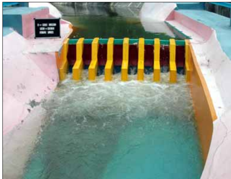
Flow Conditions for Gated Operation of Spillway for Q=9938 \text{ m}^3/\text{s}
