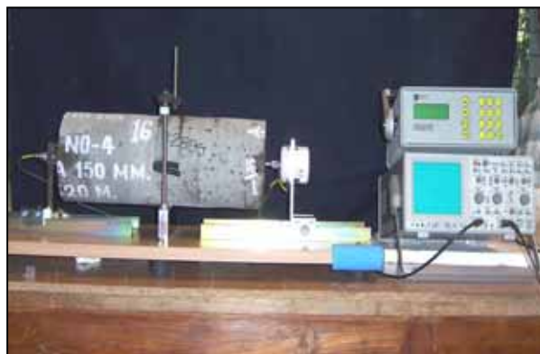
Test Setup for Determination of Dynamic Modulus of Elasticity
