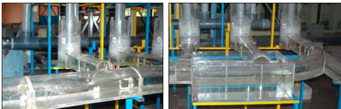
Flow at the Junction of Unit TRT I and Collection Chamber for the Condition of All Units Operational for the Original Design
