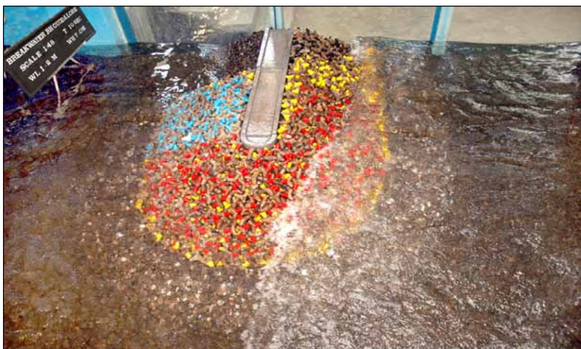
Testing Roundhead in Diffraction Basin of Wave Flume
