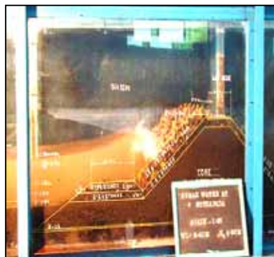
Flume Studies for Action of Random Waves ( H_s = 6.8 m) at HWL
