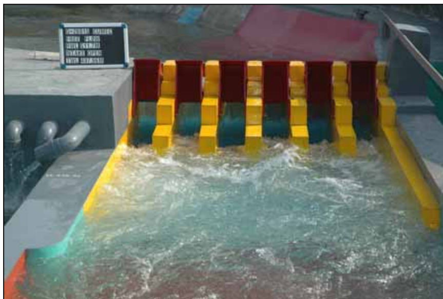
Performance of Stilling Basin for Un-Gated Operation of spillway for Q=26615 \text{ m}^3/\text{s}
