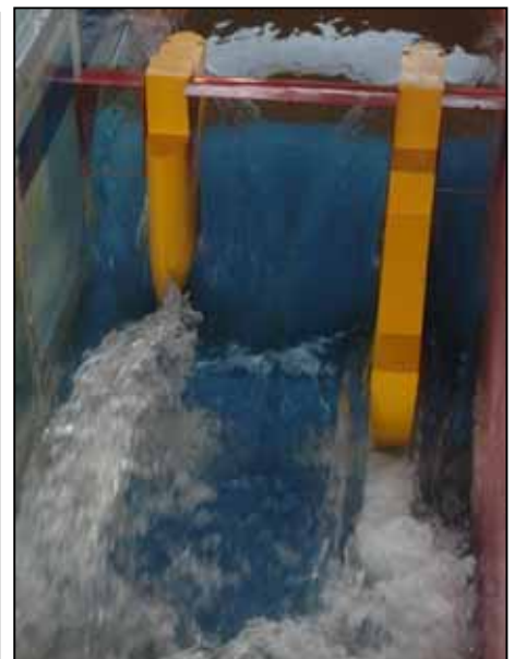
Flow Condition for Discharge of 3,500 m 3 /s
